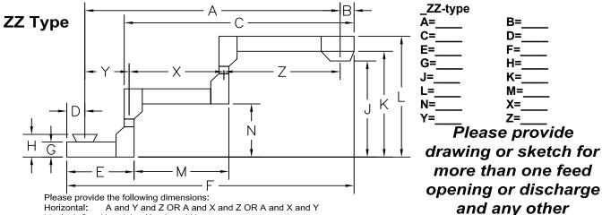
Horizontal: A and Y and Z OR A and X and Z OR A and X and Y Vertical: G or H and J or K or L and N All other dimensions are optional
